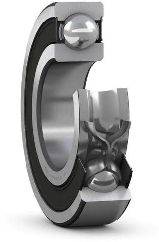
Single row deep groove ball bearings with seals or shields are particularly versatile, have low friction and are optimized for low noise and low vibration, which enables high rotational speeds. They accommodate radial and axial loads in both directions, are easy to mount, and require less maintenance than many other bearing types. The integral sealing can significantly prolong bearing service life because it keeps lubricant in the bearings and contaminants out.
